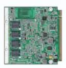
Qseven module based on Intel® Atom™ E640T/ E660T/ E680T platform with DDR2 SDRAM, four PCI Express lanes, 24bit LVDS, SDVO,CAN bus, NANDrive
