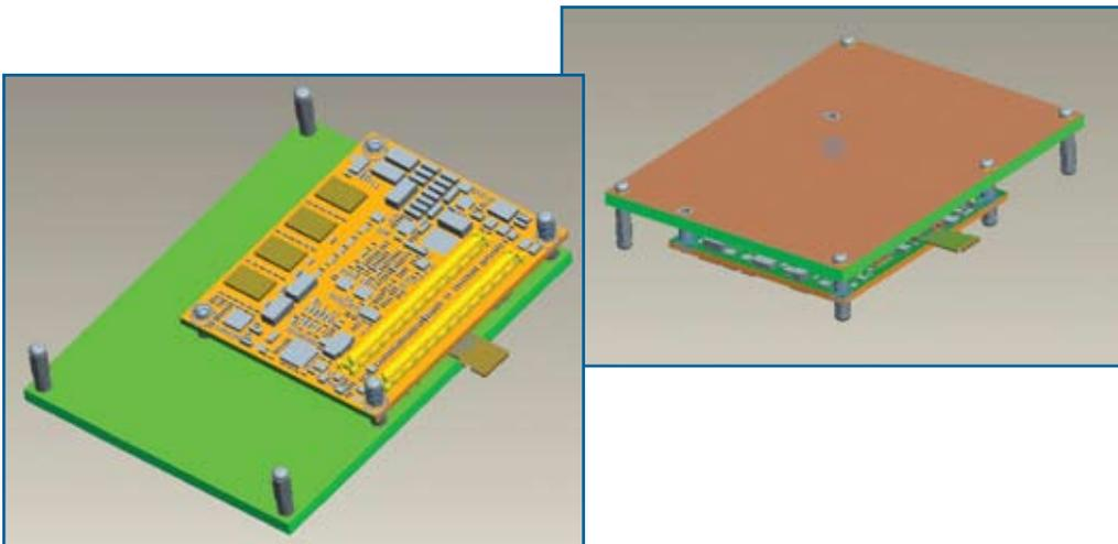
**Figure 1:** Heat-spreader provides mounting site specifically for Procelerant Z500 module and doubles as an adapter to Basic Form Factor mechanical footprint, enabling use of the new module with existing COM Express designs.
